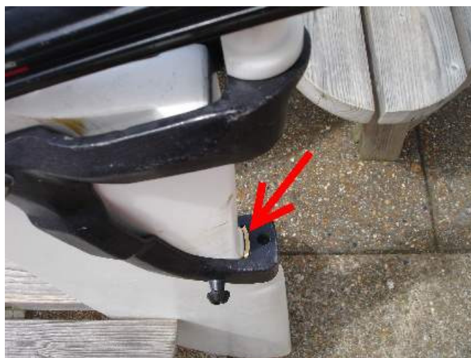
Illustration 1: Rudder blade vertical and snug against stock leather spacer
