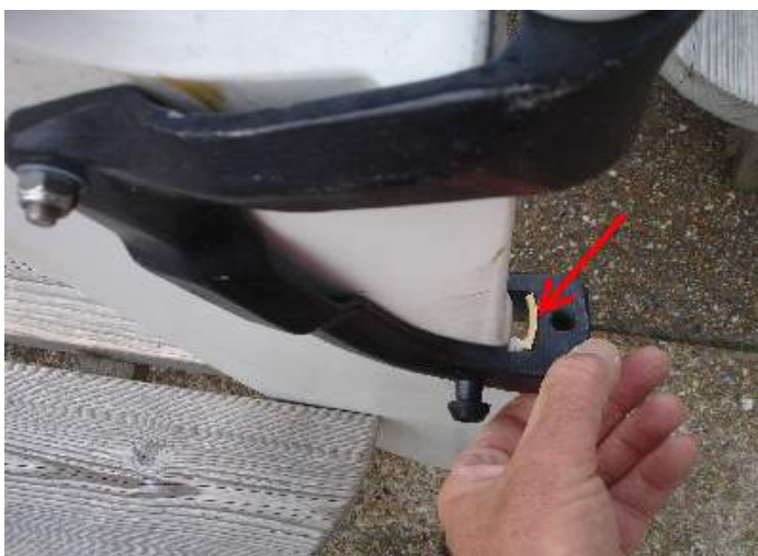
Illustration 2: Rudder blade NOT fully vertical
